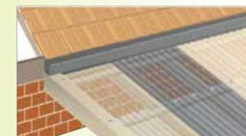
**UNDER A GUTTER** - Fit Back channel flashing with foam infill strips under gutter prior to laying sheets and Barge Capping to edge of sheet.
