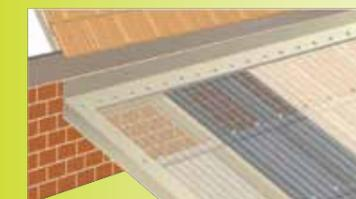
**AGAINST A WALL/FASCIA** - Fit barge capping to edge of sheet and apron flashing at the wall or fascia. Secure using recommended fixing screws.
