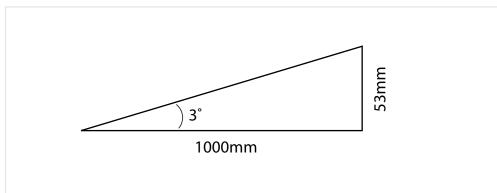
• To ensure proper water runoff, slope should be at least 3° (53mm rise over 1m length).
